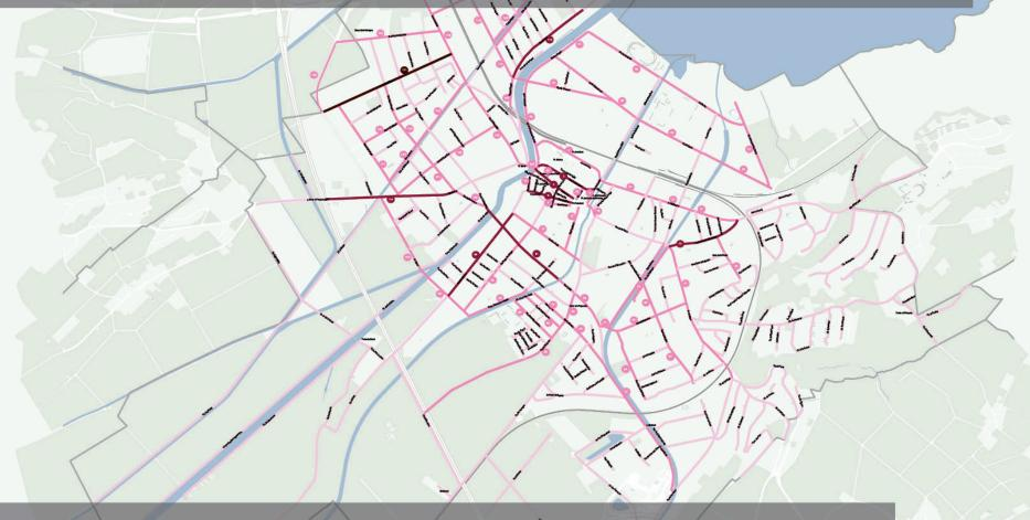
The **network analysis** is a method that allows to analyze the hierarchy relations between streets, identifies the crucial nodes, establishes the degree connection between the areas of the city.
